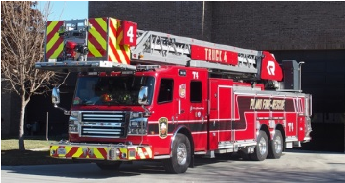
Truck 4 - 2014 Rosenbauer / Waterus 1250 GPM Pump, 300 Gallon Tank, 101 Foot Aerial Platform
