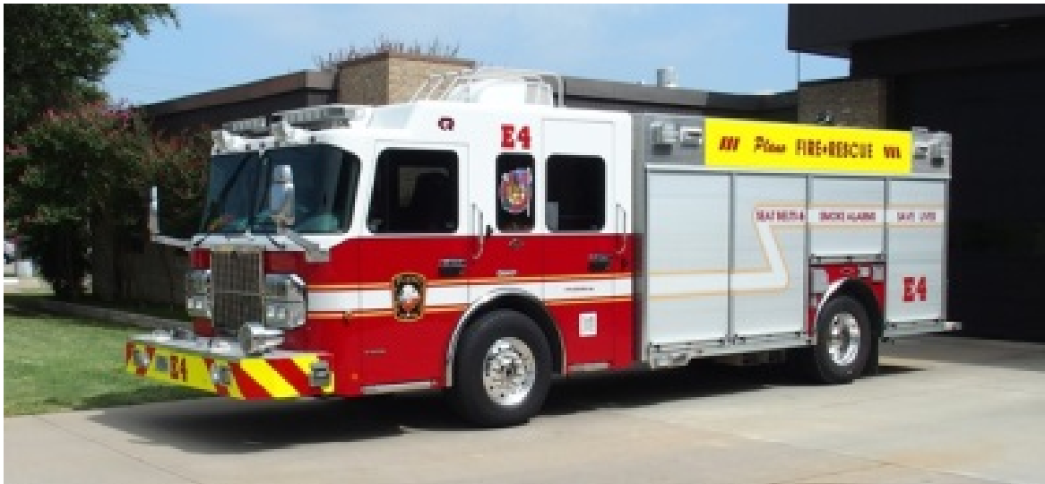
Engine 4 – 2008 Rosenbauer 1250 GPM Pump, 500 Gallon Tank, CAFS
