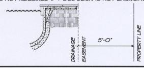
EXAMPLE 3' WHEN ANY PART OF THE POOL STRUCTURE (INCLUDING THE DECK) ENCROACHES INTO THE DRAINAGE EASEMENT THEN APPROVAL FROM THE ENGINEERING DEPARTMENT IS REQUIRED. BUILDING INSPECTION WILL FORWARD REQUIRED POOL PLANS TO THE ENGINEERING DEPARTMENT FOR REQUIRED APPROVAL PRIOR TO ISSUING PERMIT.
